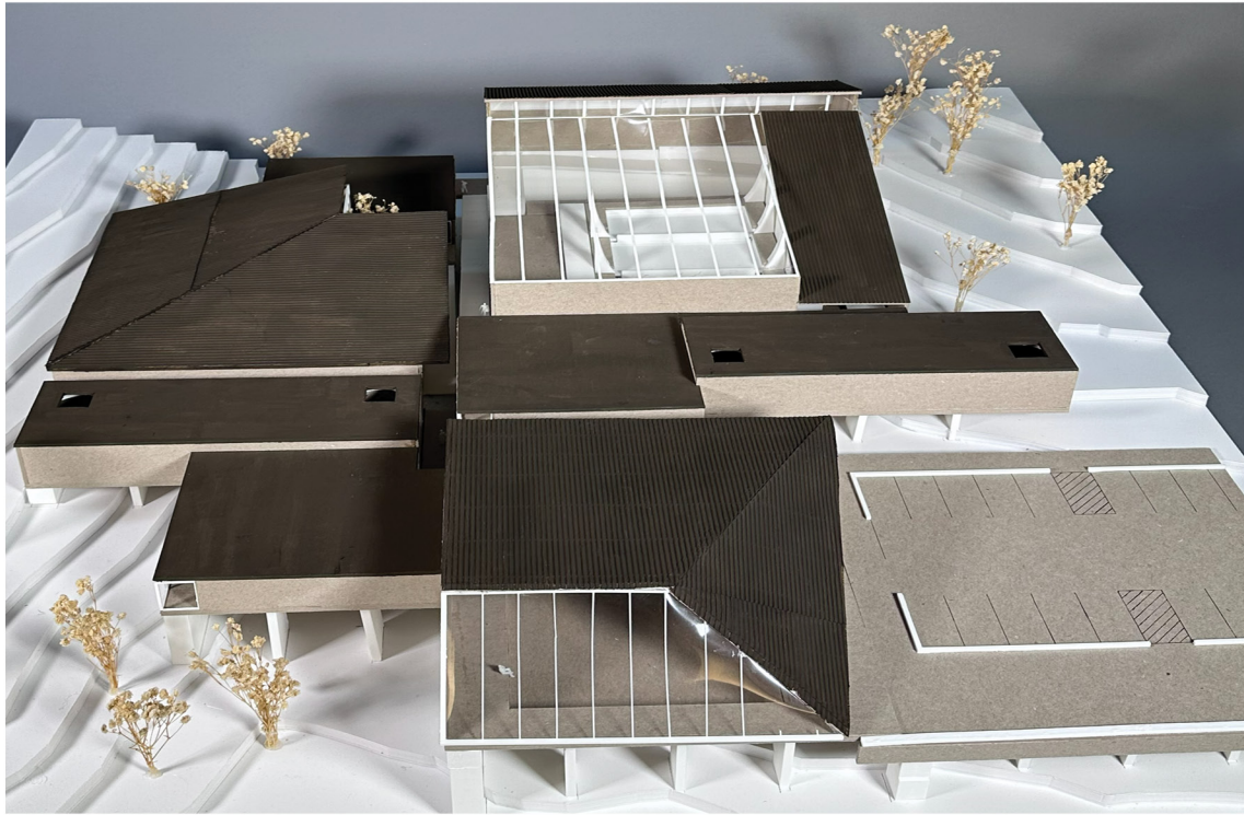
1/8" Scaled Model. Constructed with chipboard, foamboard, rugated cardboard, 3d prints, acetate.
